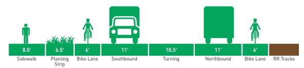
Figure 2: Existing Roadway Cross Section (looking north)
