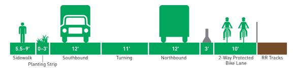
Figure 3: Proposed Roadway Cross Section (looking north)
